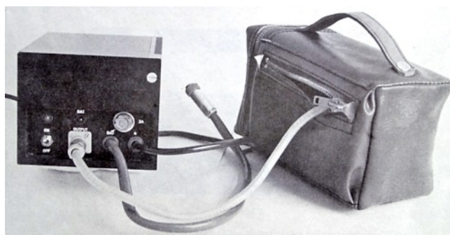
AC mains power supply unit (left) and rechargeable NiCad accumulator pack for the M-135P.
